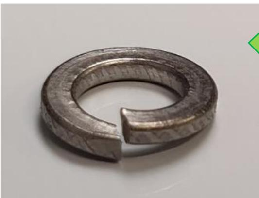
**Ensure spring washers are under every bolt head, these will take out differential thermal contraction that might otherwise cause loosening of the bolts, and thus compromise thermal contact.**
