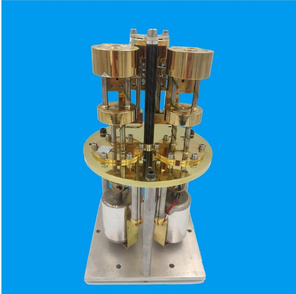
**Photo shows a typical CRC CC4 sorption cooler**
