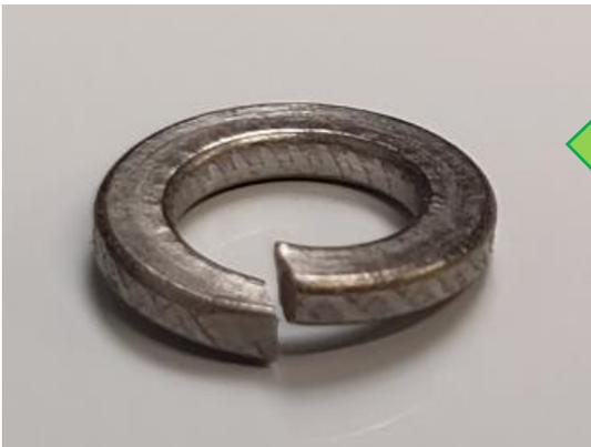
**Ensure spring washers are under every bolt head, these will take out differential thermal contraction that might otherwise cause loosening of the bolts, and thus compromise thermal contact.**
