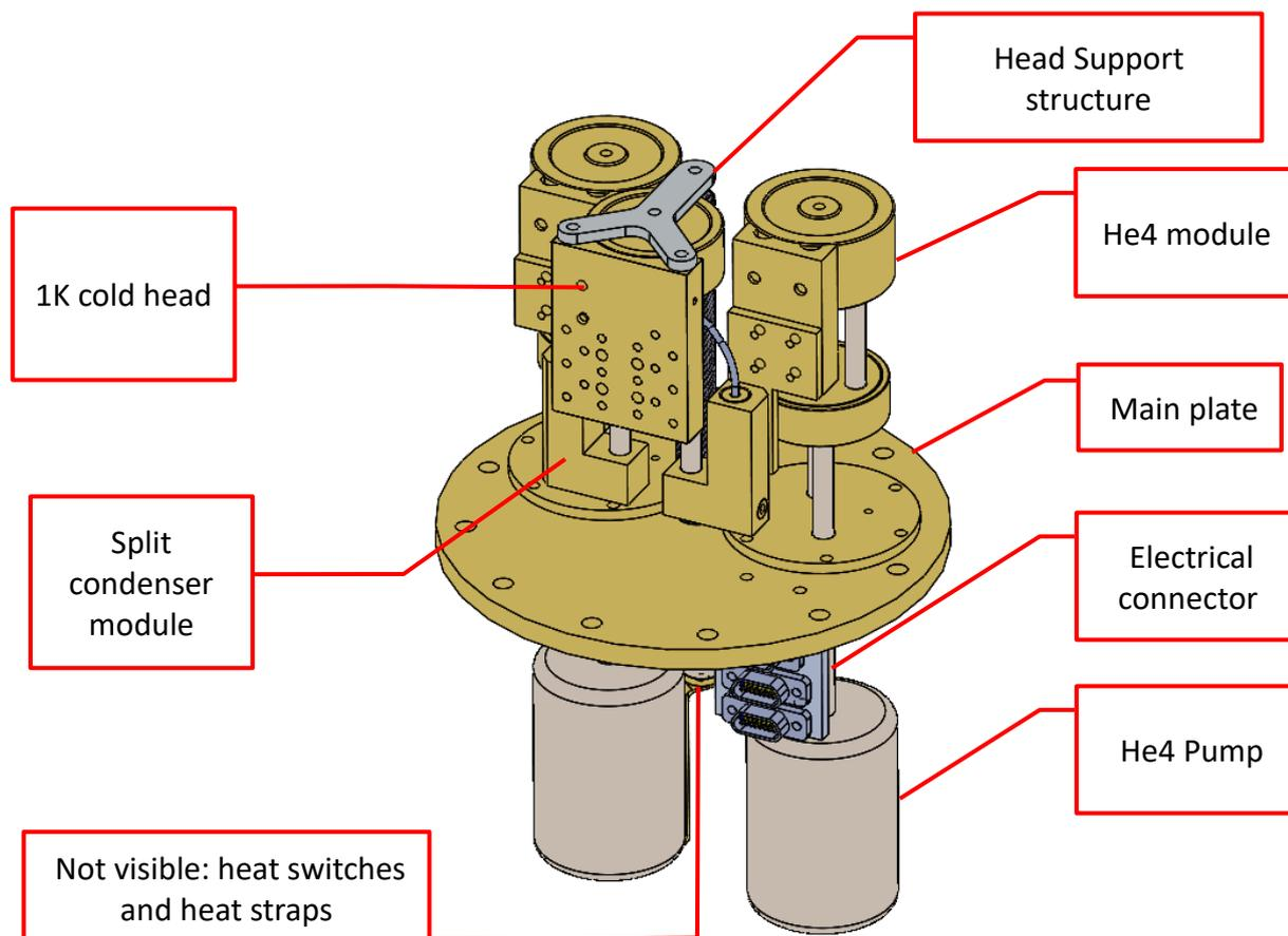
The following short names for the various parts of the sorption cooler are used throughout this user manual:
