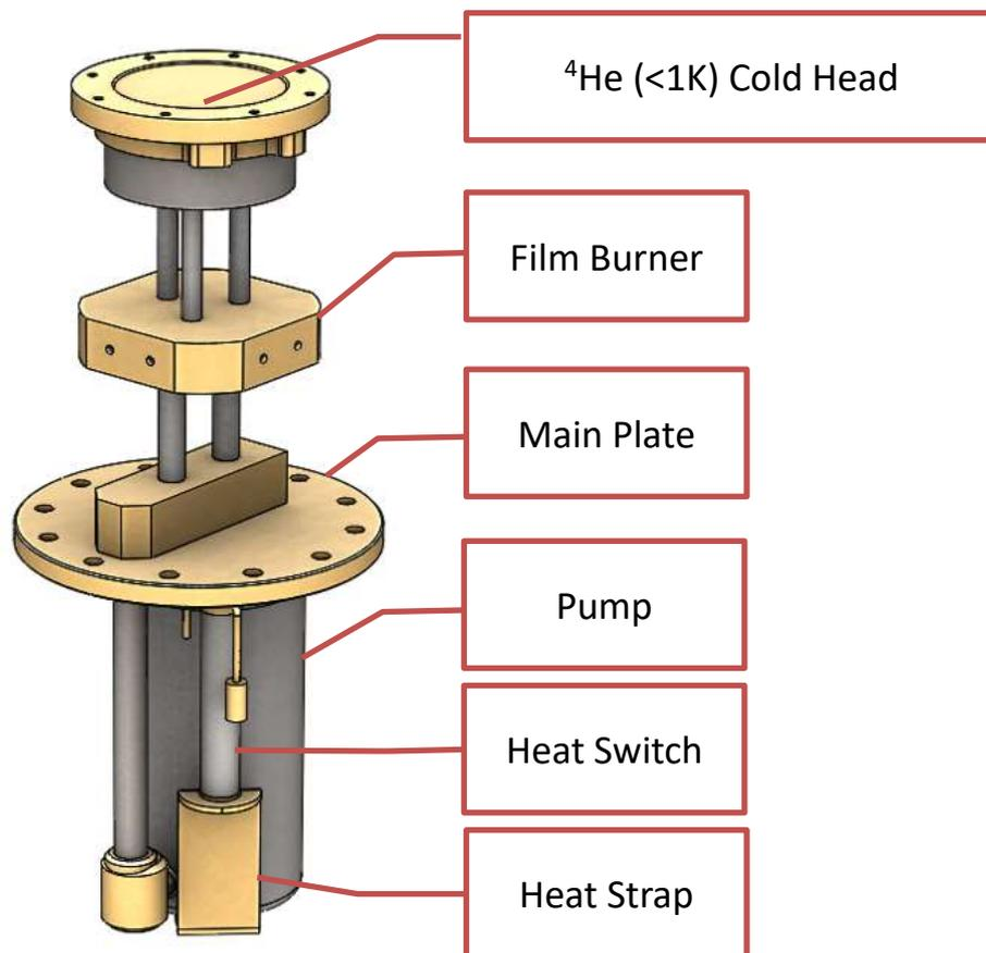
The following short names for the various parts of the cryocooler are used throughout this user manual:
