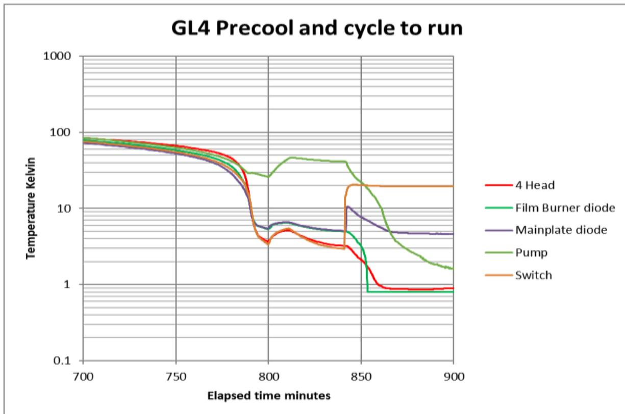
Here you can see that after  $\sim 800$  minutes the 4-head temperature is less than  $4\text{K}$ , the 4-switch is off ( $<10\text{K}$ ) and the pump is at more than  $25\text{K}$ . To get the GL4 running the pump is warmed to  $\sim 45\text{K}$  by applying a voltage of  $20\text{V}$ . The pump heater is turned down or off while the head temperature drops
