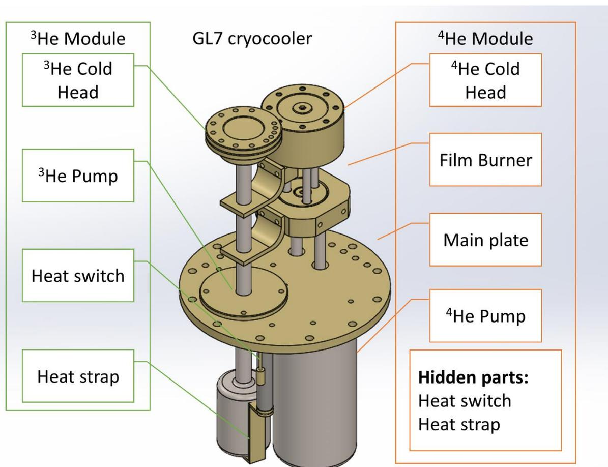
The following short names for the various parts of the cryocooler are used throughout this user manual:
