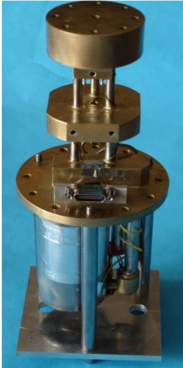
**Photo shows a typical CRC GL4 cryocooler**
